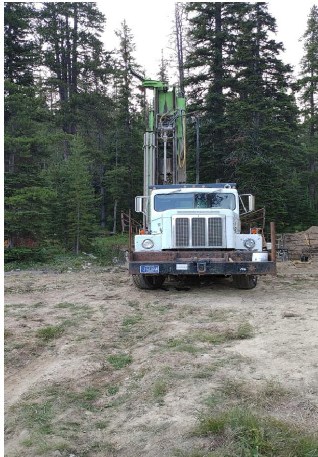
Figure 1: Reverse Circulation Drilling Rig Set up to drill Golden Jubilee Vein
