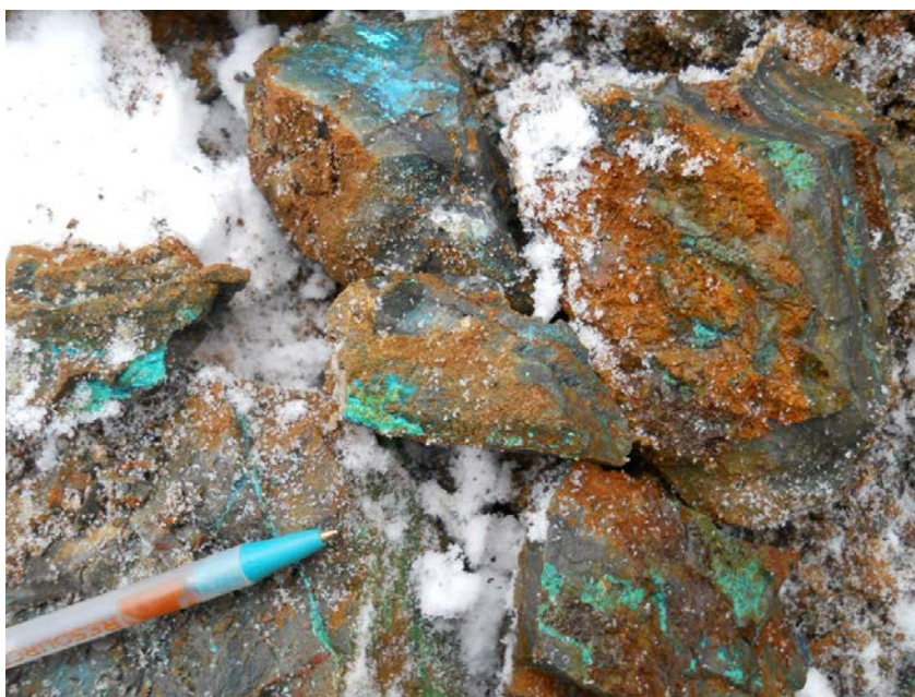
Photo 5: Cu-oxide stained siderite-altered rocks on the Richmond Adit waste dump, UTM607579-5243192
